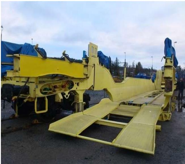
Fig. 1. Specialized wagon in the ready position for loading [4]
