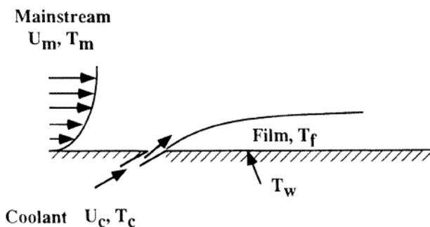
Figure 3 Schematic of film cooling concept
