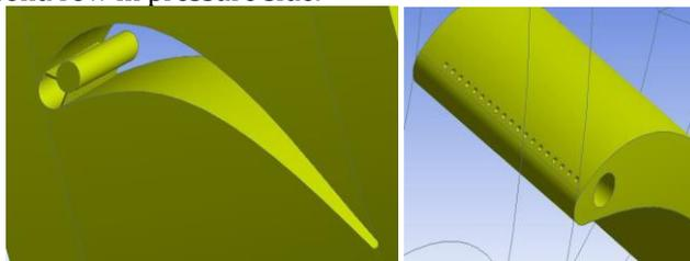
Figure 9 Location and orientation of holes 19 x 15 x 25mm
