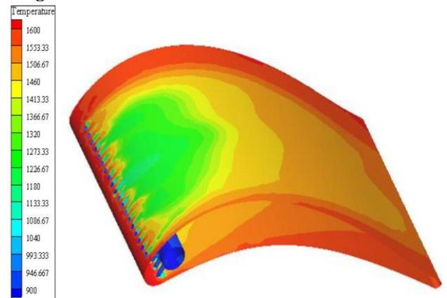
Figure 13 Temperature contour on Blade surface at Suction Side
