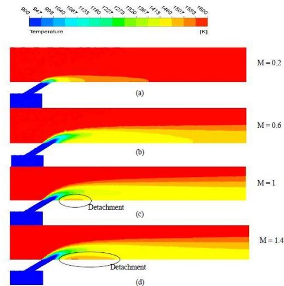
Figure 6 Film flow at various blowing ratios
