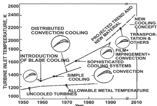
Figure 1 Year wise improvement in Inlet temperature respective with the different technologies
