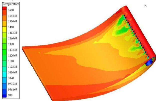
Figure 14 Temperature contour on Blade surface at Pressure Side
