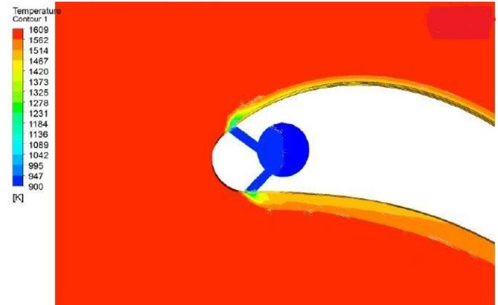
Figure 12 Film of cooling air over a Blade surface
