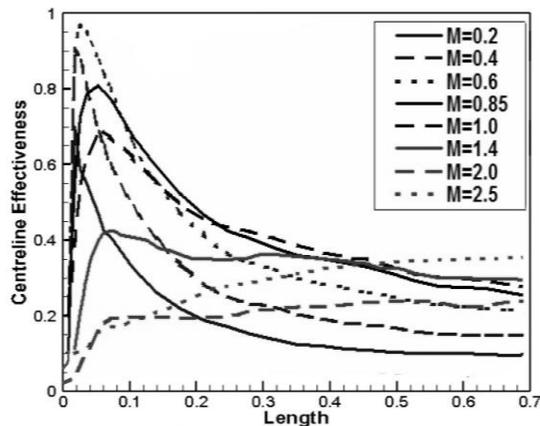
Figure 7 Plot of Centreline Effectiveness to the length in flow direction for various M.
