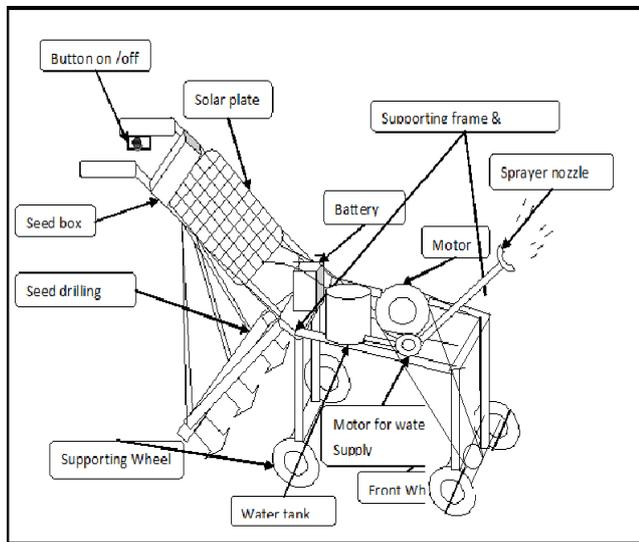
Fig. Schematic block diagram of solar operated multipurpose agriculture robot
