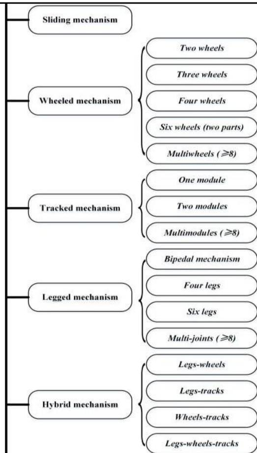
specifying the major subsystems and their possible solutions based on functional analysis (Such as the functional tree method). The investigation of an adaptable and energetically autonomous climbing robot for indoor applications is the aim of on-going research in Loughborough University.
