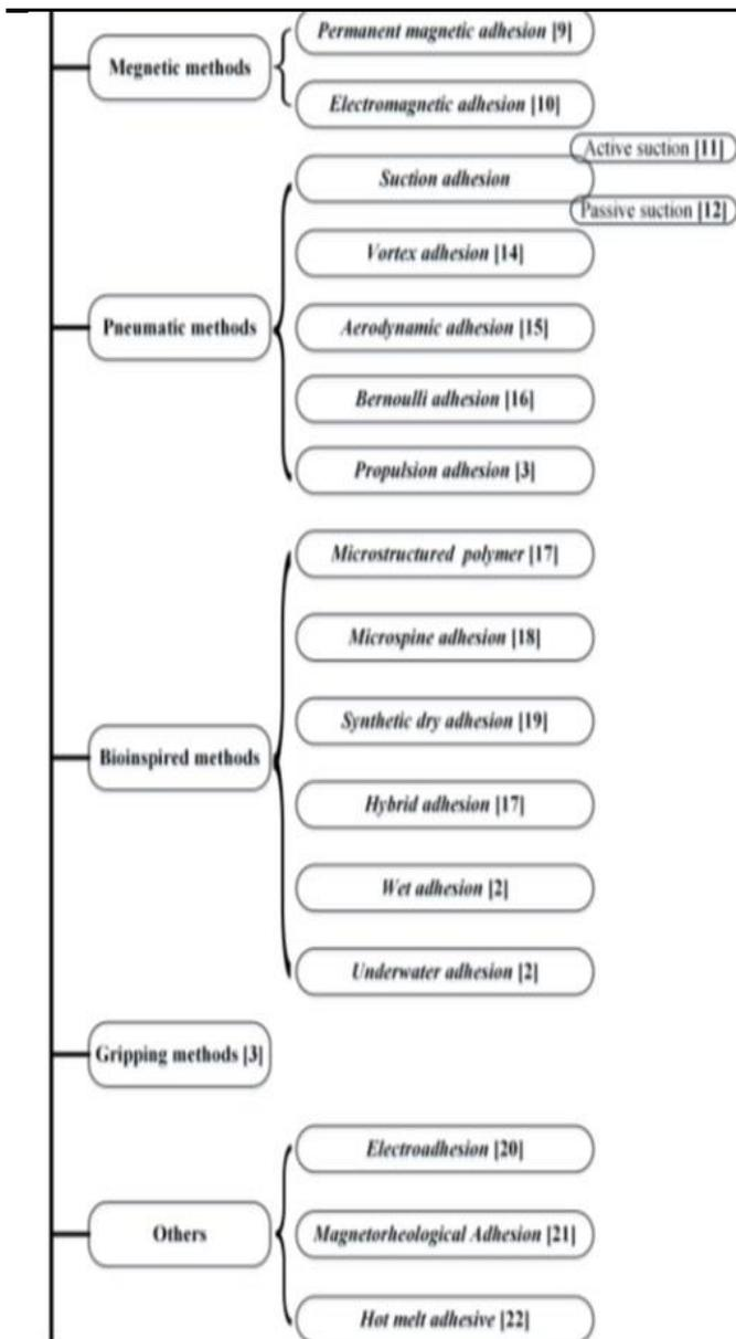
Fig. 1 Adopted adhesion methods in climbing robots
