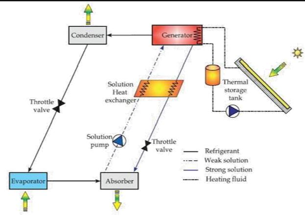
Fig. 2: Schematic Diagram Of Solar Absorption Refrigeration System[2]
