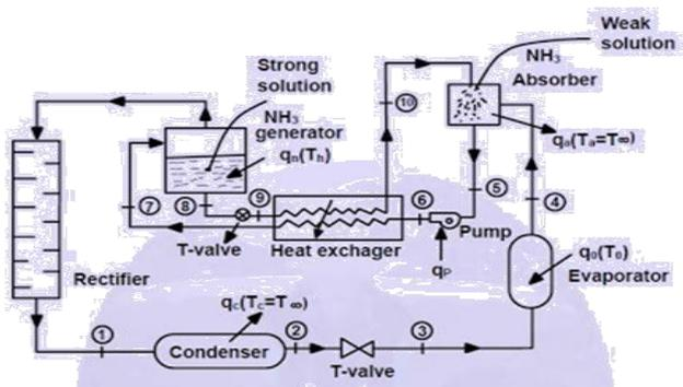
Fig. 1: Schematic Diagram of Vapour Absorption Refrigeration System.[7]
