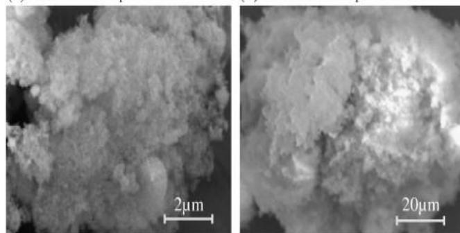
Fig. 2: Nano-aluminium powders and Micro aluminium powders [4]
