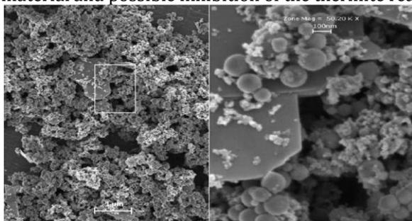
Fig. 1: SEM images of 80-nm Al particles mixed with MoO<sub>3</sub> particles.[19].
