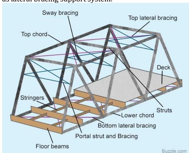
Fig 3: Lateral Bracing for Truss Bridges
