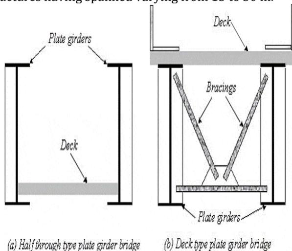
Fig.1: Deck Type Plate Girder Bridge
