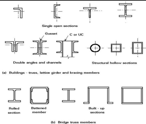
Fig 2 : Typical Cross Sections For Truss Members
