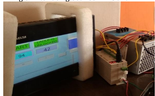
Fig.7: Interfacing between PLC and HMI
