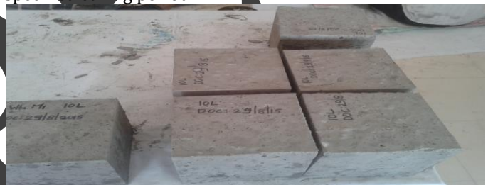
Figure 1. Specimen with Lime addition cured at normal room temperature
