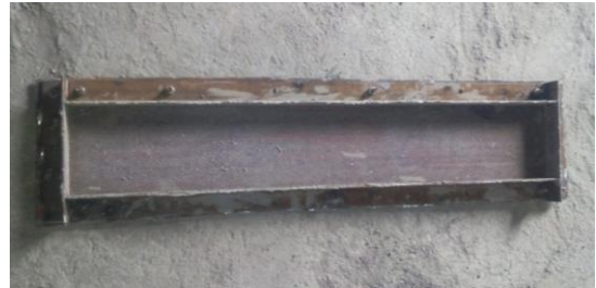
Figure No. 1. Sample Mould for Casting
