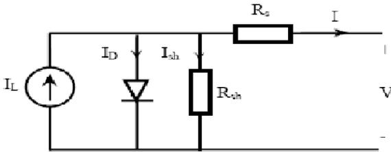
The model contains a current source, one diode, internal shunt resistance and a series resistance which represents the resistance inside each cell. The net current is the difference between the photo current and the normal diode current is given by the equation.
