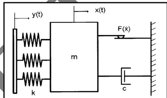
**Fig.No.3 Schematic diagram depicting a S.D.O.F oscillator with viscous, Coulomb friction and base excitation [1]**
