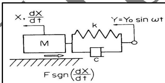
**Fig.No.2 Forced vibratory system with Coulomb friction [6]**
