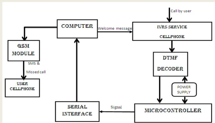
Fig -2: IVRS block diagram
