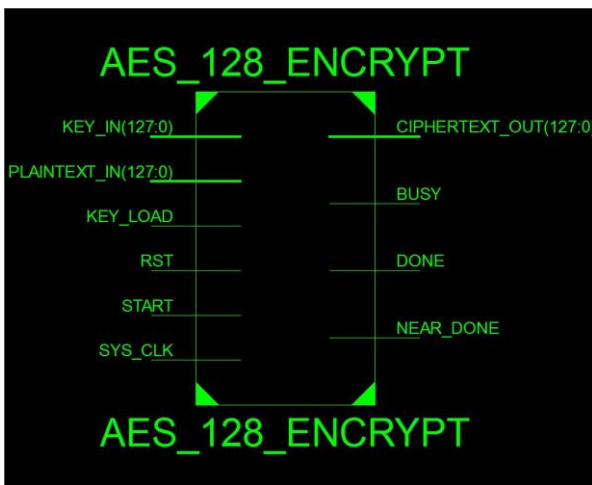
Fig. 3. The RTL schematic symbol Of AES
