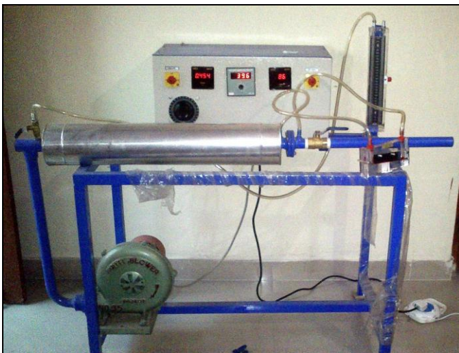
Figure 1: Experimental set up for forced convection
