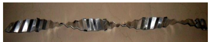
Figure 4 (a) : Aluminium corrugated insert TR-9.375, WW-13 mm
