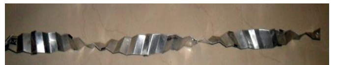
Figure 5(b) : Aluminium corrugated insert TR-9.375, WW-16 mm
