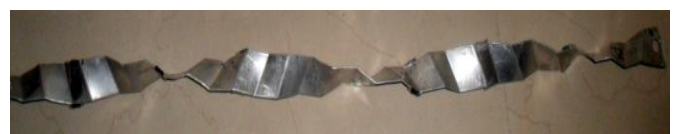
Figure 6 (c): Aluminium corrugated insert TR-9.375, WW-24 mm
