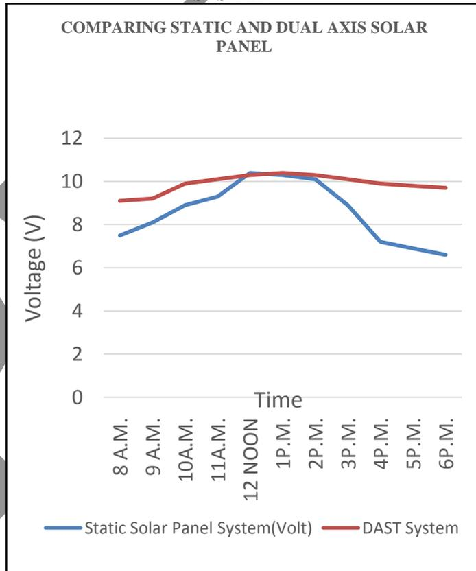
Fig.9: comparison between static solar panel and DAST system
