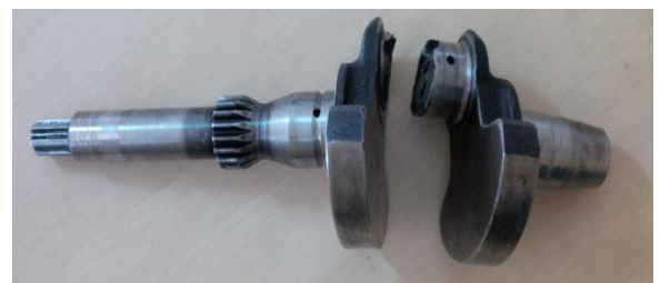
Fig. 1 Final failure On fillet of crankshaft
